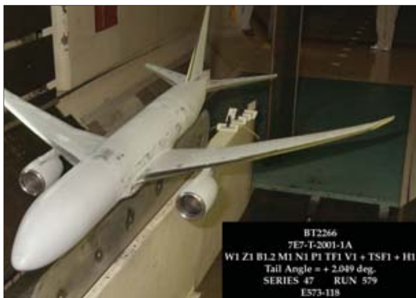
The first round of high-speed wind tunnel testing for the Boeing 7E7 was recently completed. Four different wing configurations were tested during the effort. Additional wind tunnel tests will continue through 2006.
